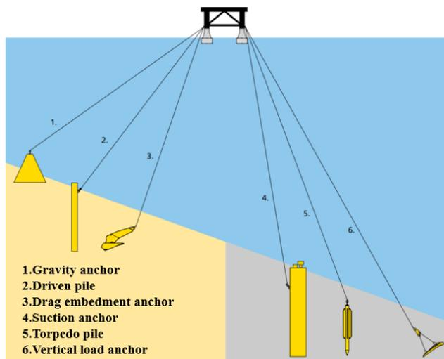
Figure 13. Typical mooring anchors <sup>[9]</sup>
