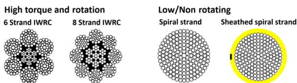
Figure 11. Various types of wire ropes<sup>[7]</sup>
