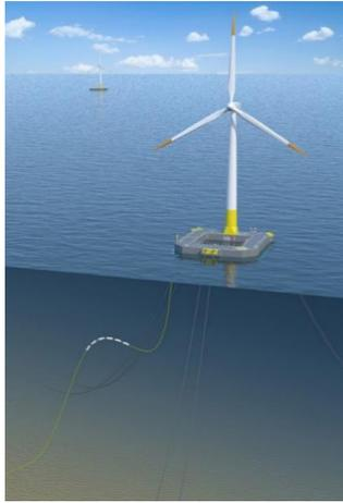
**Figure 6.** Floatgen and its mooring system <sup>[18]</sup>
