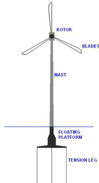
**Figure 7.** Sketch of FWT with tether mooring <sup>[20]</sup>
