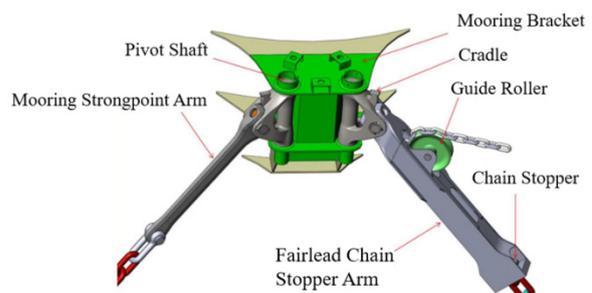
Figure 3. Hywind Scotland fairlead chain stopper system<sup>[11]</sup>
