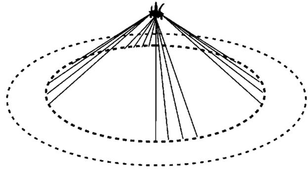
**Figure 5.** The taut mooring system <sup>[9]</sup>
