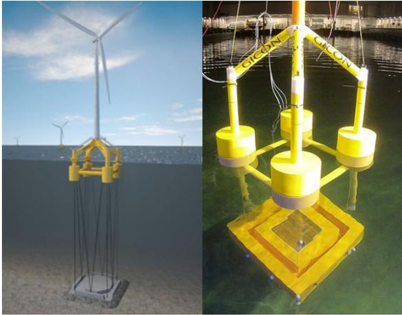
**Figure 8.** GICON-SOF project (left) and its model test (right) <sup>[26]</sup>
