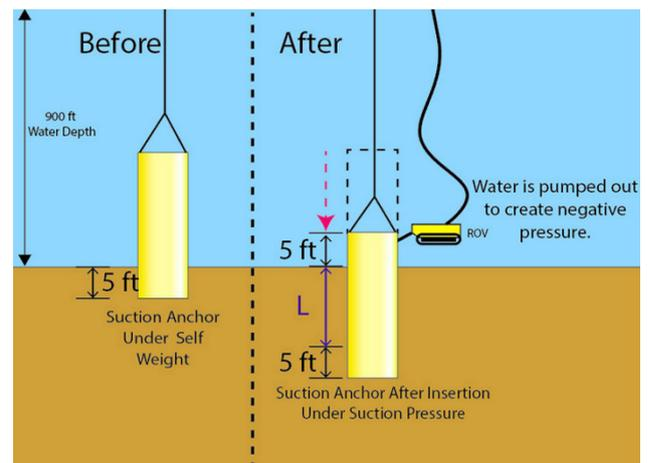
Figure 14. Installation process of the suction anchor <sup>[36]</sup>
