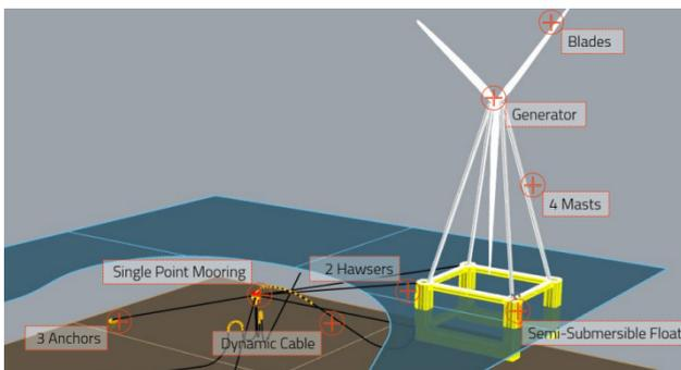
**Figure 9.** Eolink with single-point mooring <sup>[27]</sup>
