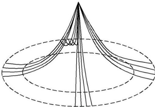
Figure 1. The catenary mooring system<sup>[9]</sup>
