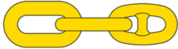
**Figure 10.** Stud-less chain (left) and stud-link chain (right) <sup>[9]</sup>
