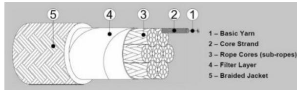
Figure 12. Composition of a synthetic fiber rope<sup>[31]</sup>
