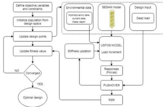
**Figure 3.** Integrated USFOS-MATLAB optimization framework
