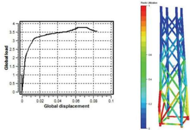
**Figure 2.** Typical load deflection curve for reference case
