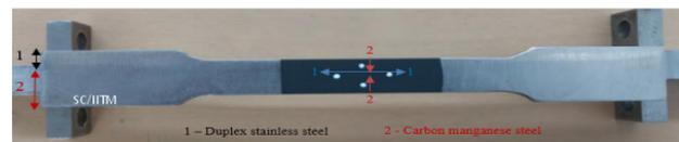
Figure 6. FGM build extracted from the specimen.
