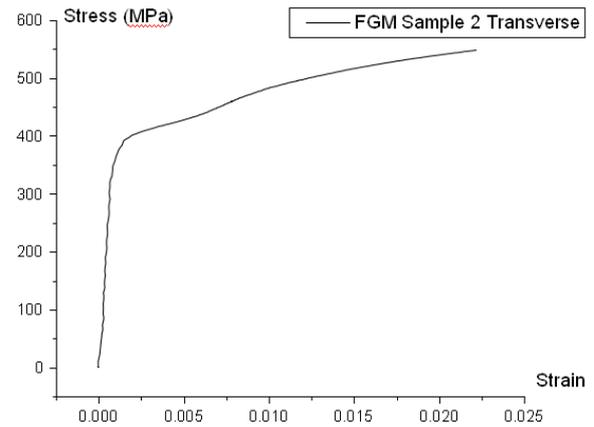
**Figure 8.** Stress-strain relationship of FGM
