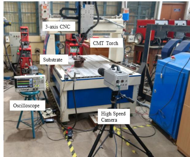
Figure 4. WAAM unit used to manufacture FGM.
