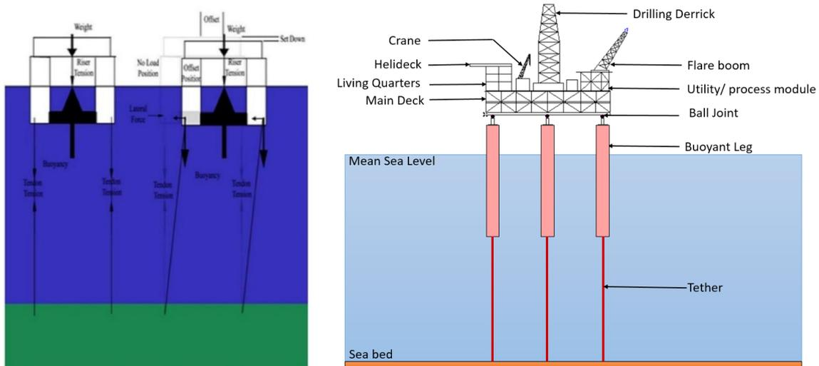
Figure 2. TLP mechanics
