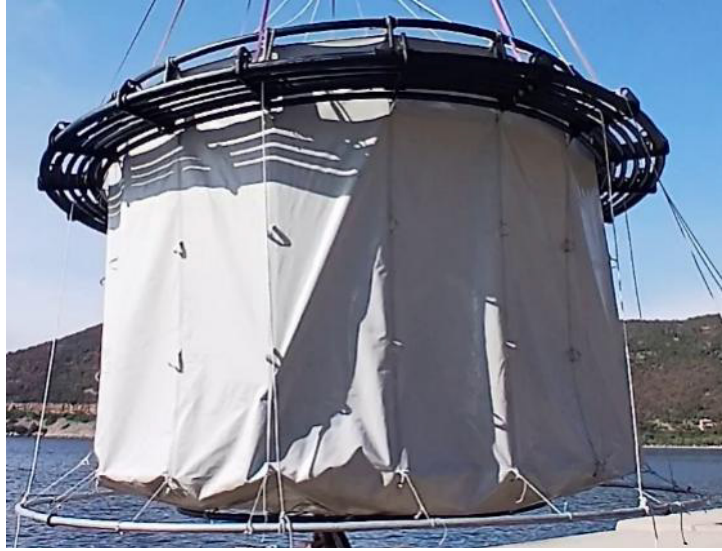
Figure 13. Mode 3 of the tank at the test location, the simplest of the three modes where all wall reinforcing ribs and vertical guides have been removed.
