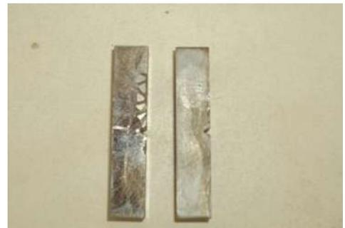
Figure 1. (f) 20µm Samples of Ni and Cr corroded for 2400 hours.
