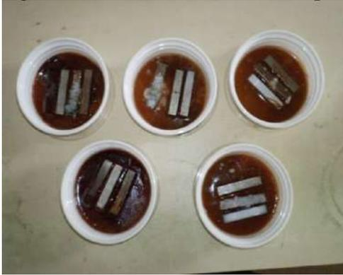
Figure 1. (c) Samples corroded in 3.5% NaCl
