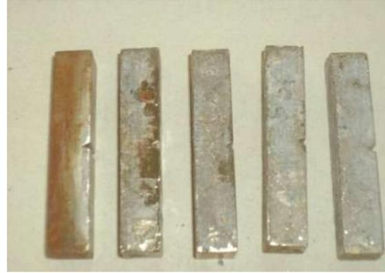
Figure 1. (g) from left to right: uncoated sample of aluminum, 6µm Ni coated aluminum, 20µm Ni coated aluminum, 40µm Ni coated aluminum and 60µm Ni coated aluminum after corroding for 2400 hours
