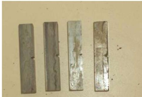
Figure 1. (e) 6µm Coated samples of PVD and electroplated samples corroded for 2400 hours
