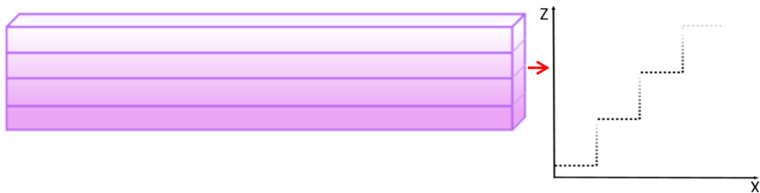
Figure 18. Stepwise gradation in the thickness (transverse) direction.
