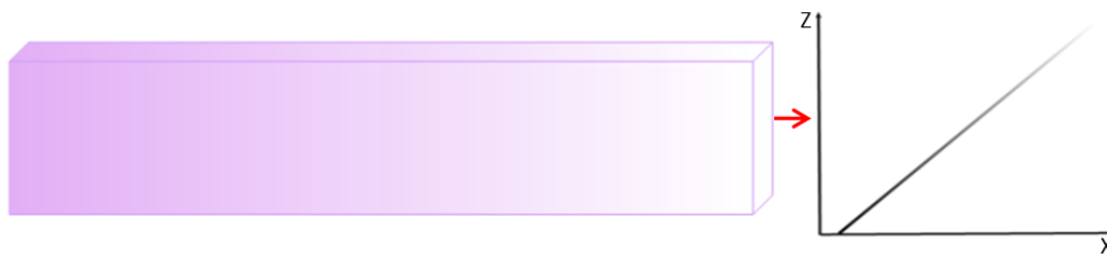
Figure 19. Continuous gradation of material property across the longitudinal direction.
