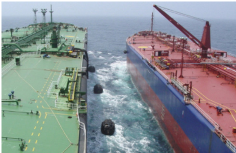
Figure 21. Ship to Ship Transfer at Sea / Anchorage using Yokohama Fenders.
