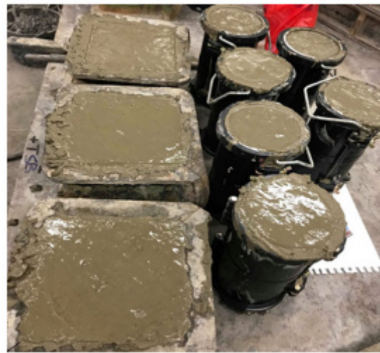
Figure 7. Bio-based concrete cubes and cylinder casting [20] .
