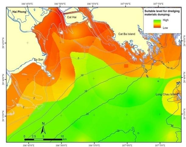
**Figure 3.** Zones of suitability for dredged material dumping
