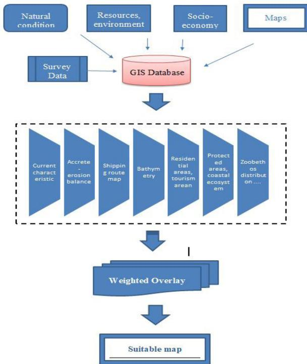
**Figure 2.** Multi-criteria GIS overlay analysis for zoning marine area of dredged material disposal
