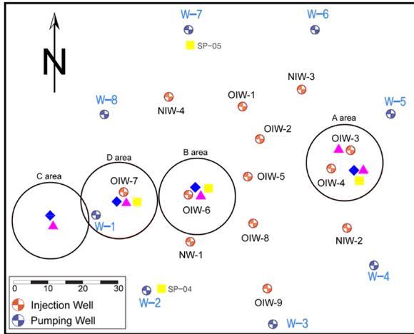
**Figure 2.** Layout of field monitoring instrumentations (modified after DAU, 2017<sup>[11]</sup>).
