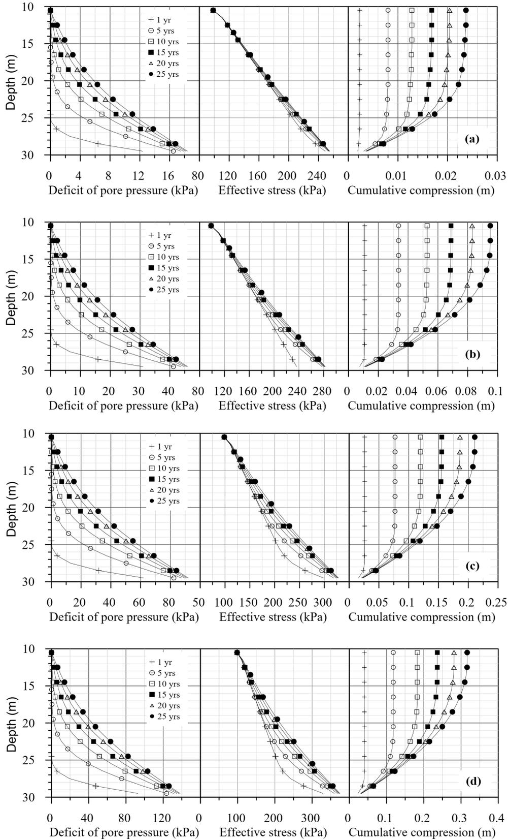
**Figure 8.** Results of 25-year consolidation analysis for the clay layer located from 10 to 30-m deep with  $C_v = 2 \text{ m}^2/\text{y}$  and different drawdowns: (a) 2.0 m; (b) 5.0 m; (c) 10.0 m; (d) 15.0 m.
