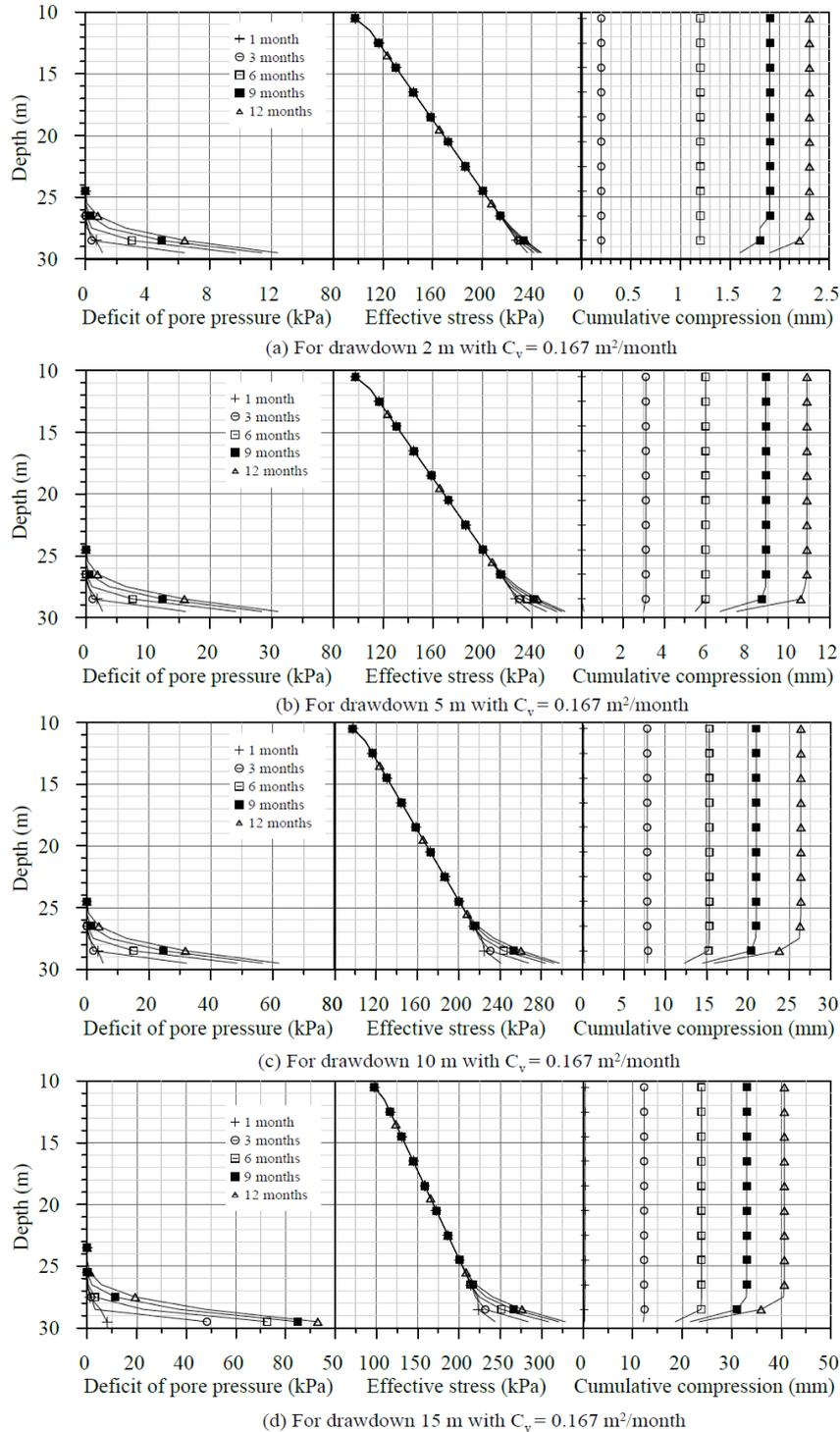
**Figure 7.** Results of 1-year consolidation analysis for the clay layer located from 10 to 30-m deep with  $C_v = 2 \text{ m}^2/\text{y}$  and different drawdowns: (a) 2.0 m; (b) 5.0 m; (c) 10.0 m; (d) 15.0 m.
