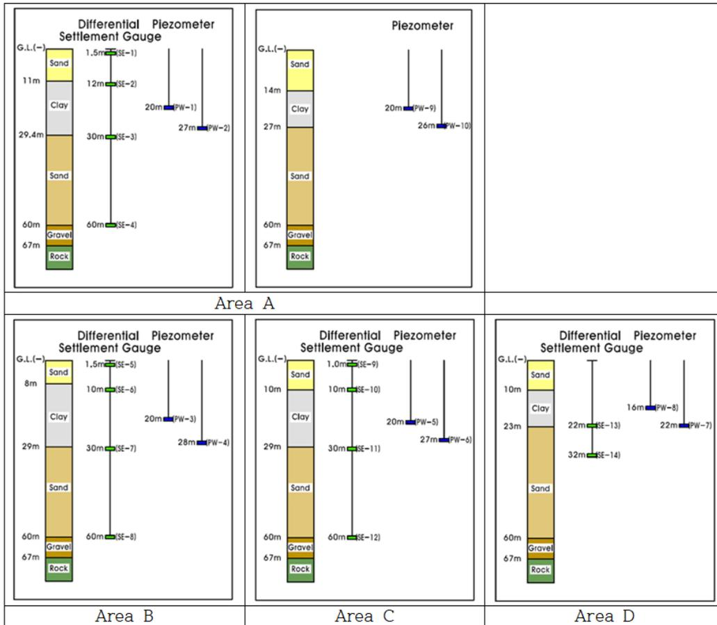
**Figure 3.** Subsoil profile and field instrumentations layouts at five monitoring areas<sup>[11]</sup>.
