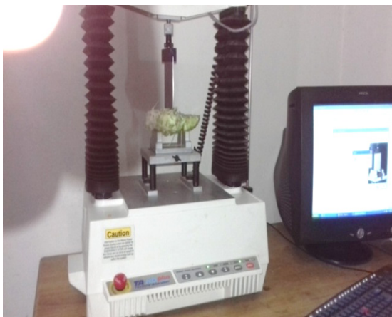
Figure 2. Measurement of stem cutting force using Texture Analyzer
